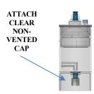
Attach clear non vented cap to the bottom port.
